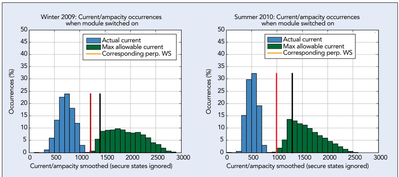
Histograms of the occurrences of actual loads and allowable dynamic load ratings. The vertical red line represents the 1,200-A static rating, and the black line is the operator target maximum of 1,400 A. It is obvious that this line has considerable capacity that is both unused and available.
