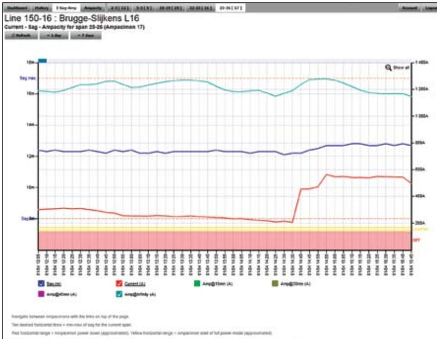
Evolution of sag and ampacity during tests in Belgium (150-kV Brugge-Slijkens line). Static rating is 613 A.
